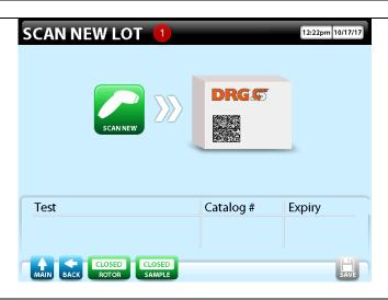
For a new assay or in case the assay version was changed, the Assay Protocol Barcode (APB) has to be scanned. The APB is in the **Insert for Use (IFU) page 2.** The parameter information has to be loaded in the instrument. Close the procedure by pressing the "SAVE" button.
