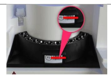
Load on board the Needle Cleaning Solution (NCS)
